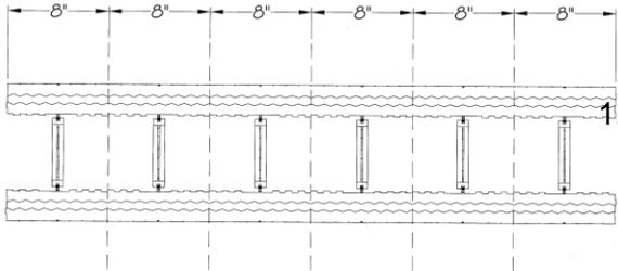
1. Cut straight panels into 8" increments. When cutting, make sure you keep the web centered in the 8"
