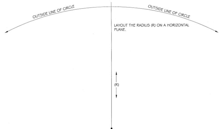
3. From the center of the circle, snap a chalk line extending beyond the mark for the outside of the radius.
