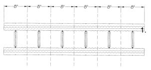
1. Cut straight panels into 8" increments. When cutting, make sure you keep the web centered in the 8"
