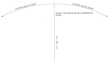
Mark the outside of the radius on the footing or slab. If site conditions do not permit the radius to be marked on the footing or slab, any horizontal surface will do.
