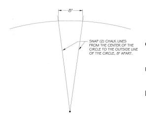
3. From the center of the circle, snap a chalk line extending beyond the mark for the outside of the radius.
